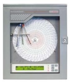
Sentinel's high speed chart advance / reverse facility allows the chart to be set quickly to the correct time mark.
