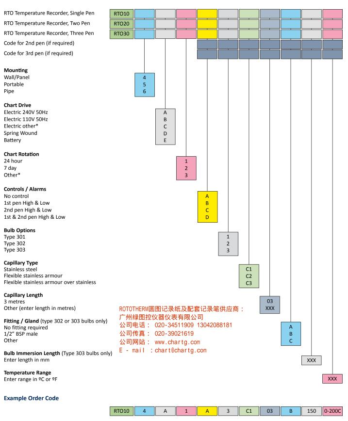
Single pen temperature recorder, wall mounted, electrical 240 volt 50hz chart drive, 24 hour rotation, no control, type 303 bulb, 3 metres of stainless steel capillary, 1/2" BSP male compression fitting, immersion length 150 mm, range 0 to 200 Deg C.
